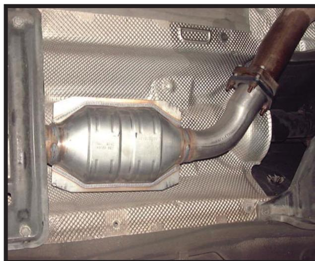
**REPAIR TIME:** The temperature a cat reaches depends to a large extent on how rich an engine is running. If the mixture is too weak or lean, the cats suffer. Pre-cat lambda sensors play a central role in maintaining this air-fuel ratio.
