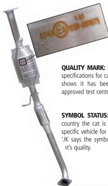
**QUALITY MARK:** R103 legislation controls the manufacturing specifications for catalytic converters. Seeing this stamp on a cat shows it has been tested by an independent government-approved test centre such as Millbrook.
